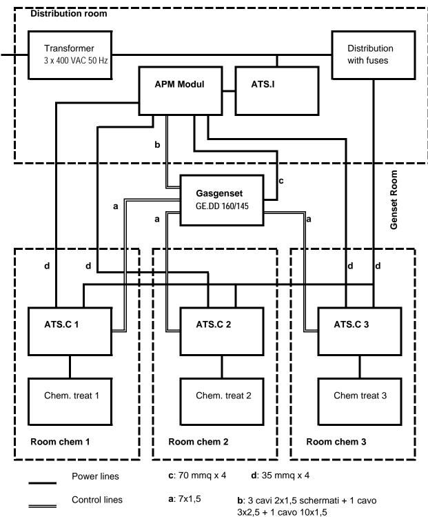
Genset has to be between the transformer and the distribution. As the distribution has fuses, which can blow, the genset has to be connected direct with 3 change over switchtes located by the chemical treating units, detecting an power inerruption.. If the chemical treatment stops, the mass will blow out explosif gases.
